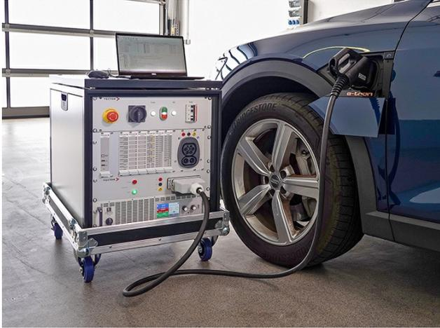
*Performing automated conformance testing using CANoe Test Package EV on a real e-vehicle (Source: Vector)*
