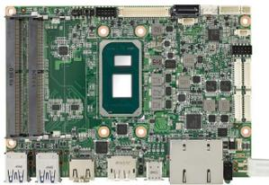
MIO-5375 SBC features the 11<sup>th</sup> Gen Intel Celeron processor, which is up to 25 % faster than its predecessor (Source: Advantech)
