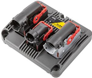
*SL84 safety controller for applications up to PL d and SIL 2 (Source: Epec)*
