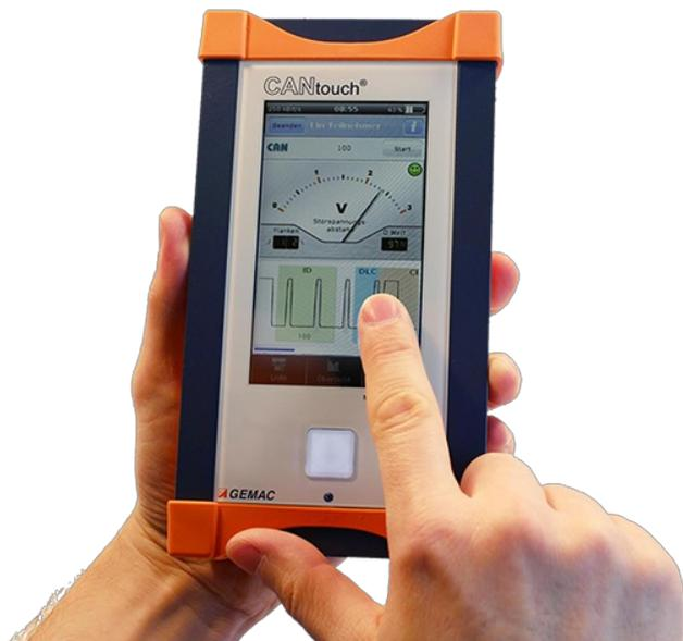
Figure 1: Fieldbus diagnostic system CANtouch (Source: Gemac)
