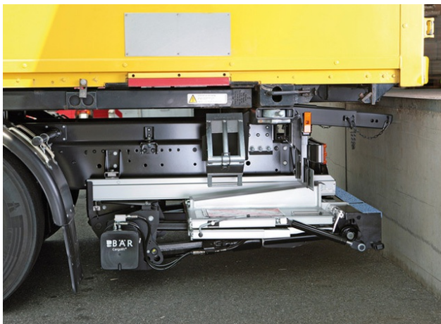
Tail-lifts are a typical body application unit, which communicate with the in-vehicle networks and a telematics gateway (Source: Baer Cargolift)
