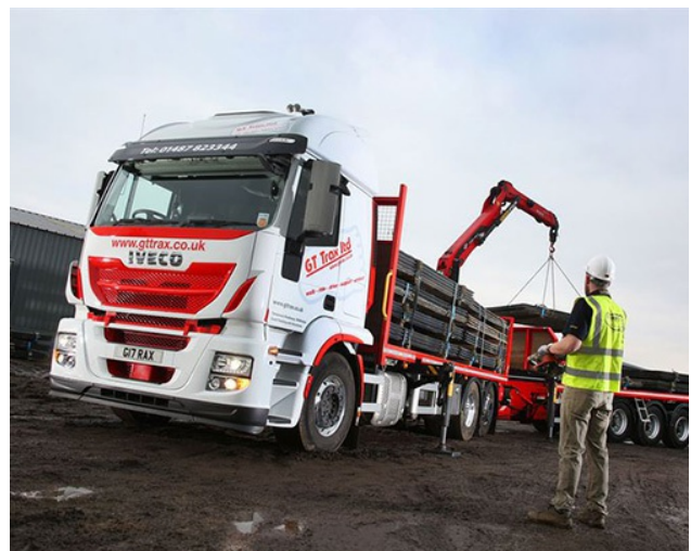
The CiA 413 profile series standardizes the interface to in-truck networks for cranes and other body applications (Source: Iveco)
