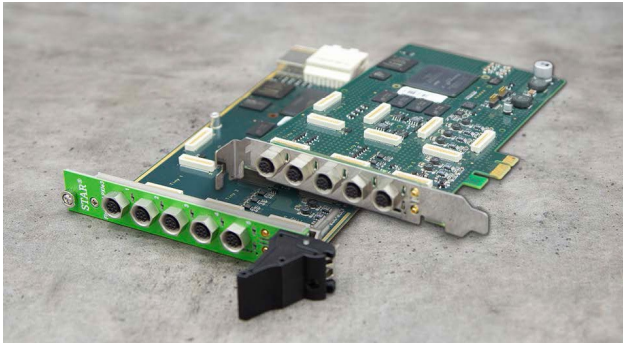
Flexcard PXIe3 and PCIe3 cards enable data acquisition from up to 30 automotive networks (Source: Star Cooperation)
