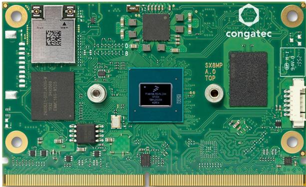
*Peripheral interfaces include 2x CAN FD, 1x PCIe Gen 3, 2x USB 3.0, 3x USB 2.0, 4x UART as well as 14x GPIO (Source: Congatec)*
