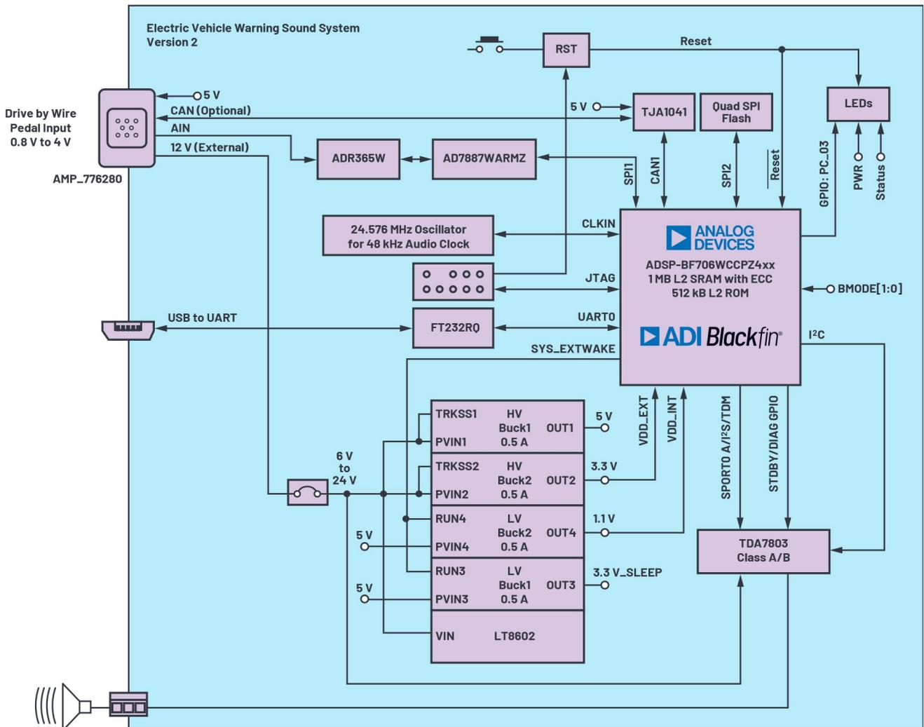
Detailed system block diagram with a Blackfin+ processor on a board with reduced components (Source: AD)
