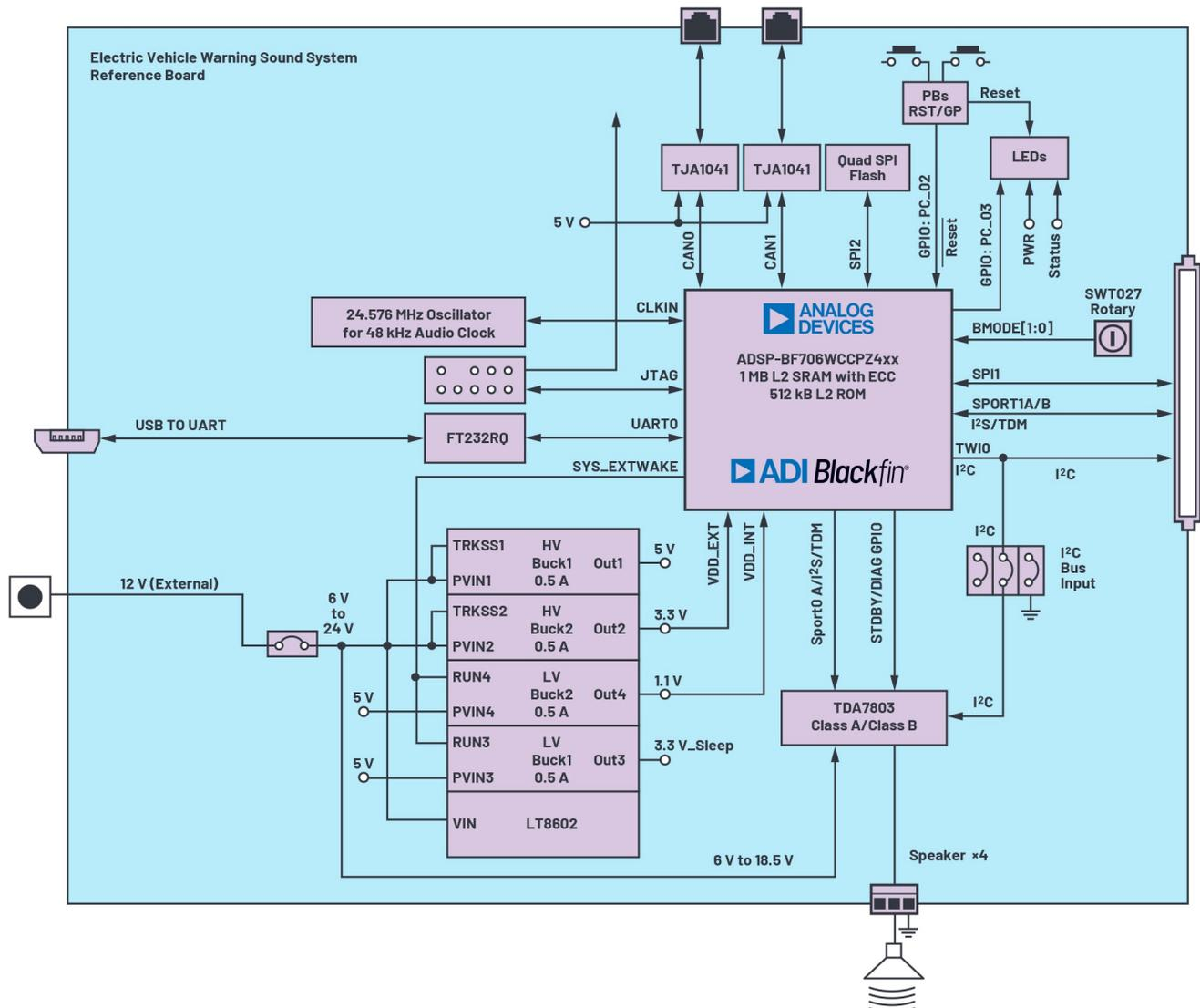
Detailed system block diagram with a Blackfin+ processor on a full-featured board (Source: AD)
