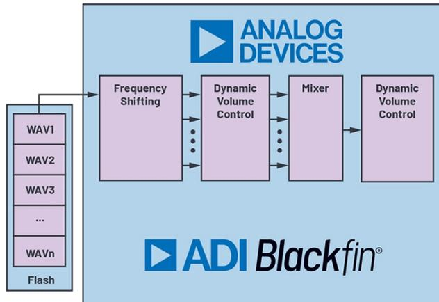
Processing blocks on Blackfin+ processor (Source: AD)
