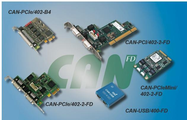
CAN FD boards of 402 series in various form factors (Source: ESD Electronics)
