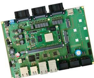
NXP announced their S32G vehicle network processor at this year's CES show. As an early adopter, Micorsys offers the Miriac MPX-S32G274A system-on-modules and development kits based on this central processing unit family. The system combines interfaces for CAN (18 CAN, two CAN FD), Flexray, LIN, and Ethernet interfaces for automotive networking.
