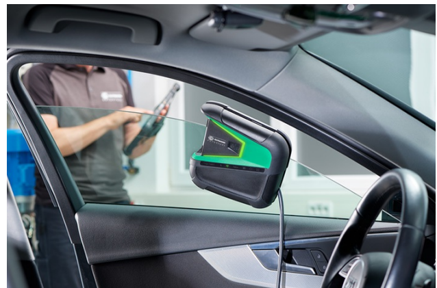
An integrated bracket allows the device to be positioned on the side window of the vehicle, thus ensuring a Wifi connection to the display/control unit, even on vehicles with chrome-plated windshields (Source: Hella Gutmann)
