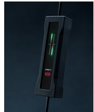
Two LED bars show the CAN traffic status including busload, error frames, and overrun (Source: Kvaser)
