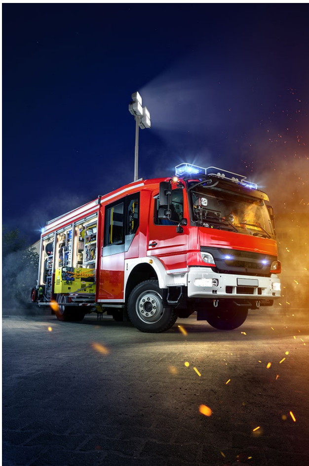
Firefighting vehicles are equipped with multiple CAN-based body-builder networks connecting specific devices (Source: Adobe Stock)
