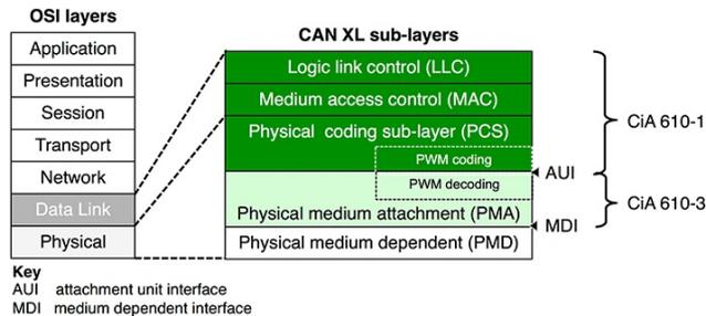
CAN XL lower layers and its mapping to the OSI model (Source: CAN in Automation)
