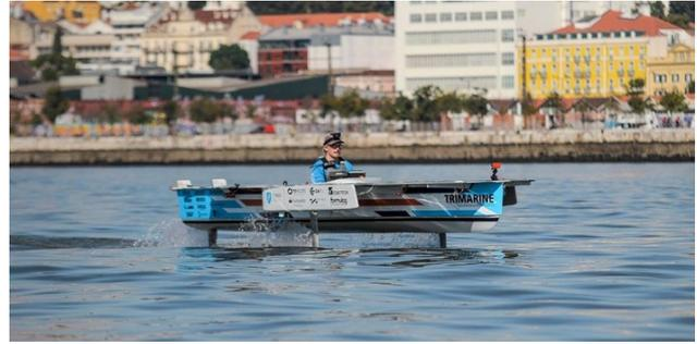
*CAN-controlled hydrofoils allow the SR02 boat to get elevated over the water line, thus reducing the drag forces and the energy consumption (Source: Kvaser)*
