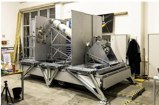
The rocket test stand for engines with a thrust of up to 24 kN (Source: Kvaser)
