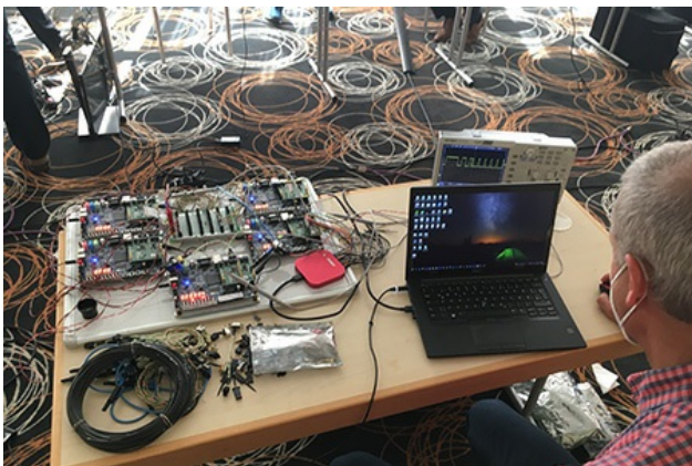
The double-star CAN XL test network by NXP comprises eight nodes (Source: CiA)
