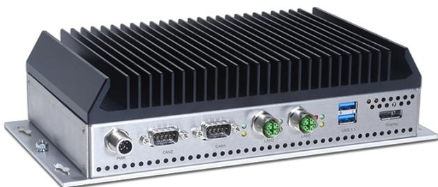
RSL A3 is designed for 24/7 railroad operation at temperatures from -40 °C to +70 °C (Source: Syslogic)
