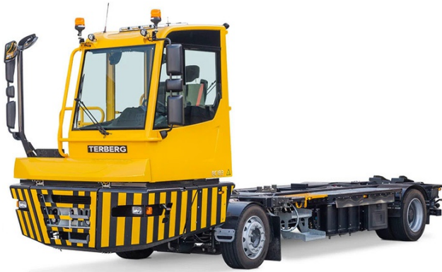
The BC183 swap body carrier. A fully electric model (BC202-EV) is also available (Source: Terberg)
