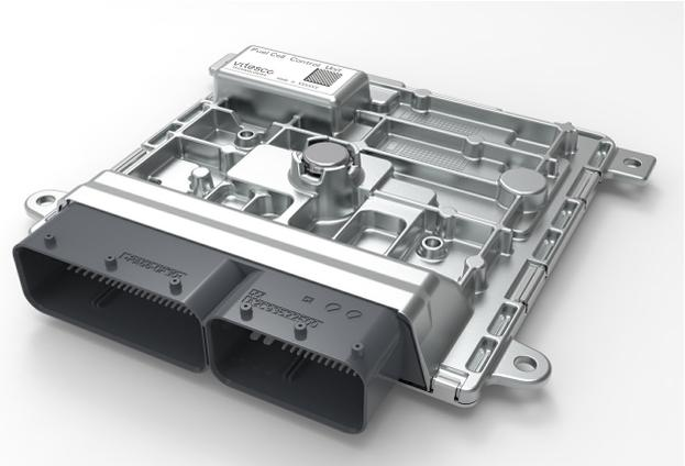
The FCCU uses CAN FD for communication within the fuel cell system (Source: Vitesco Technologies)
