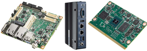
RSB-3720 single board computer (left), the EPC-R3720 box PC, and ROM-5722 computer on module (Source: Advantech)
