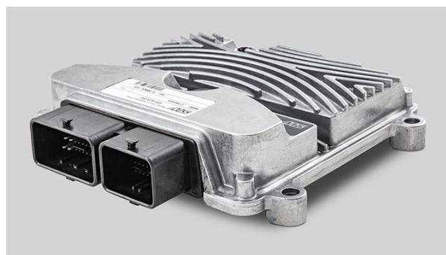
The brain of the machine: CANopen-capable control unit ESX.4cs-gw (Source: STW)
