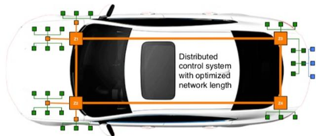
Zonal in-vehicle architecture (Source: CAN in Automation)
