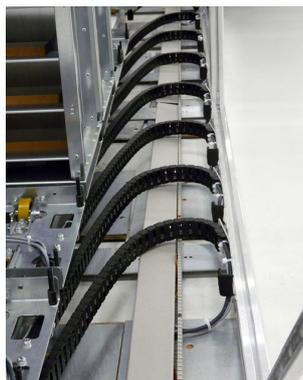
Figure 2: Each sliding cabinet receives its energy supply and signal routing from an E065 energy chain and Chainflex cables (Source: Igus)
