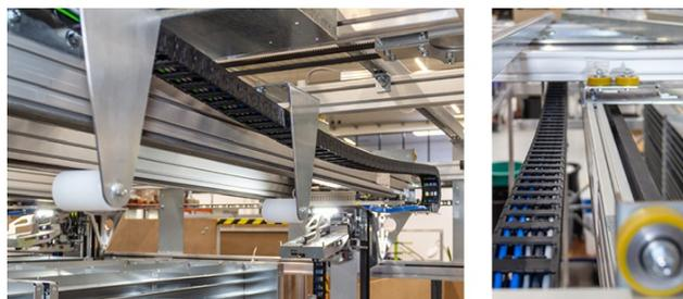
Figure 3: Energy and CAN signals reach the RBG axes through energy chains (Source: Gollmann Kommissioniersysteme)
