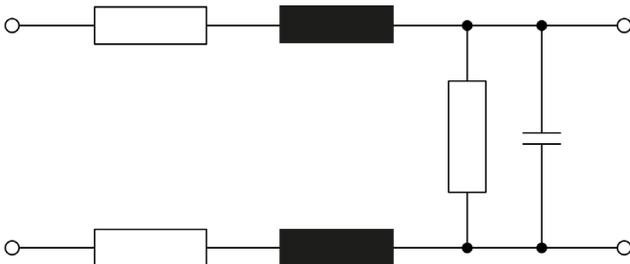
Equivalent circuit diagram of a CAN line (Source: Gemac Chemnitz)
