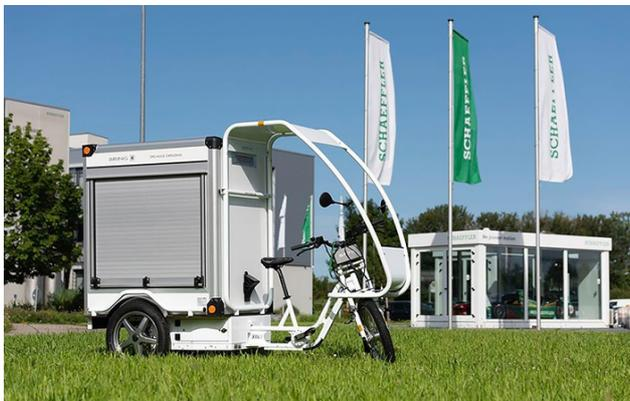
*The Free Drive operates using bike-by-wire technology (Source: Schaeffler)*
