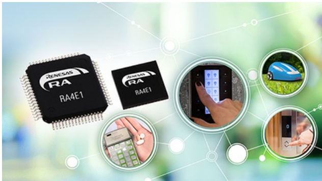
RA4E1 and RA6E1 entry-line MCUs combine low-power consumption with the 100-MHz and 200-MHz performance, respectively (Source: Renesas)
