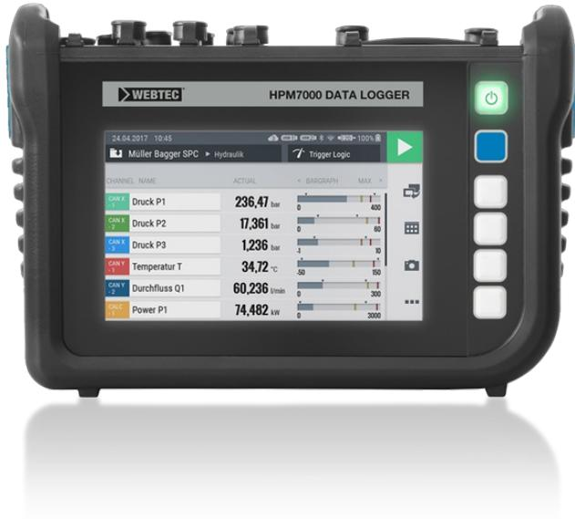
*Using the Webtec device, PDI (pre-dispatch inspection) technicians can provide a richer data set in support of machine/equipment performance prior to shipment, reducing the likelihood of end-user complaints, explained the company (Source: Webtec)*
