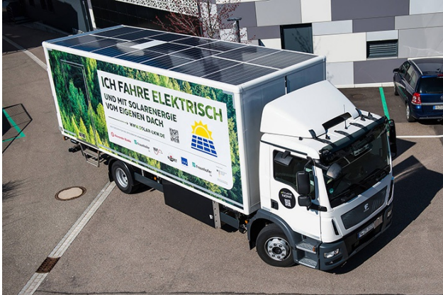
The solar modules integrated into the box body make use of the entire roof (Source: Fraunhofer ISE)
