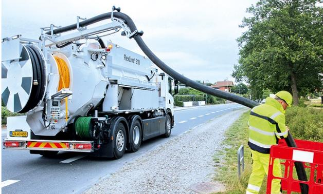
A sewer cleaning vehicle of the company Bucher Municipal with the uncoiled jetting and suction pump for sewer cleaning (Source: ifm)
