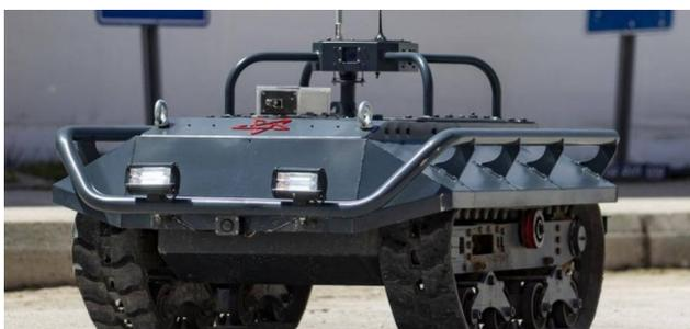
Havelsan's CAN-based unmanned ground vehicle (Source: CSS Electronics)
