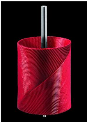
*At the heart of the DC miniature and micro-motors is the patented, self-supporting, coreless rotor coil with skew-wound design, which rotates around a fixed magnet (Source: Faulhaber)*
