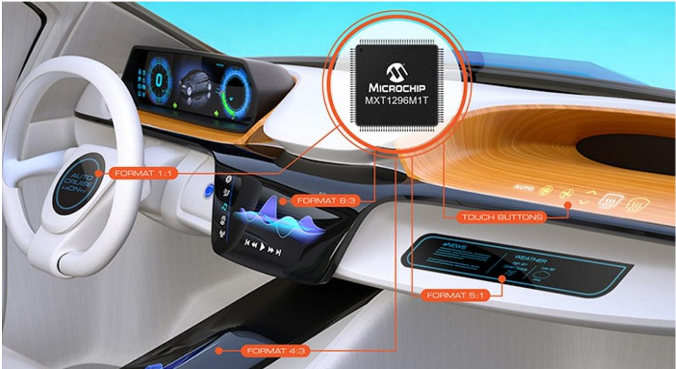
Reconfigurable driving and receiving touch channels allow to match the screen format to different aspect ratios (Source: Microchip)
