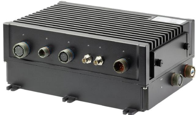
*The solution requires no fan and can be operated in an environment of -20 °C to +55 °C and comes with two CAN interfaces (Source: MPL)*
