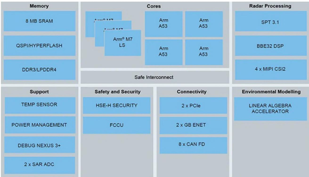
The S32R45 is equipped with eight CAN FD interfaces (Source: NXP)
