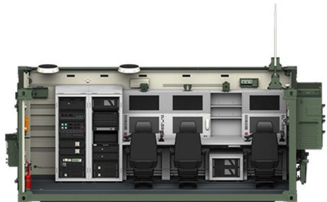
*The Byraktar TB2 drone is operated by human beings in the Ground Control Station System (Source: Baykar)*
