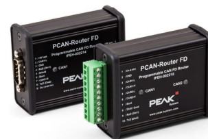
The PCAN-Router FD from Peak-System (Source: Peak/Esacademy)
