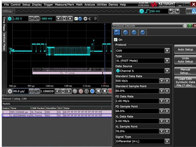
Oscilloscope screenshot of a decoded CAN XL frame (Source: Keysight)
