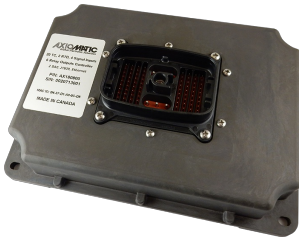
The scanner device collects data from multiple temperature sensors and sends them via a CAN interface (Source: Axiomatic)
