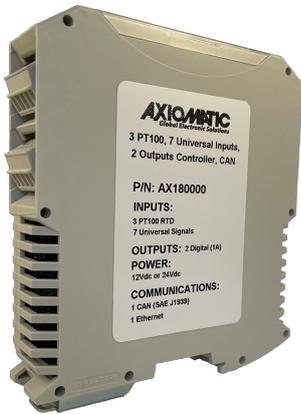
The AX1800X0 controller can be networked to J1939 (Source: Axiomatic)
