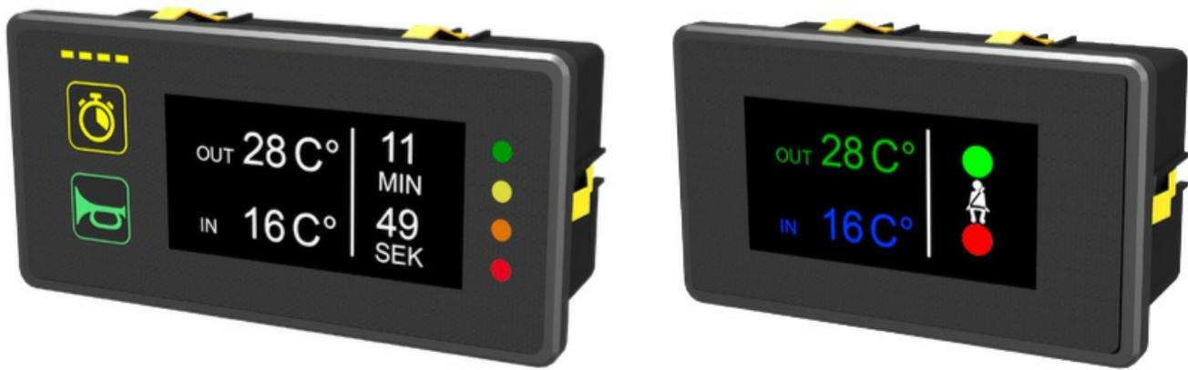
*The OLED display (left) and TFT display (right) variants next to each other (Source: Miunske)*
