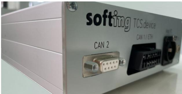
*The TCS.device is the hardware for diagnostic simulation as a replacement for real ECUs or vehicles (Source: Softing)*
