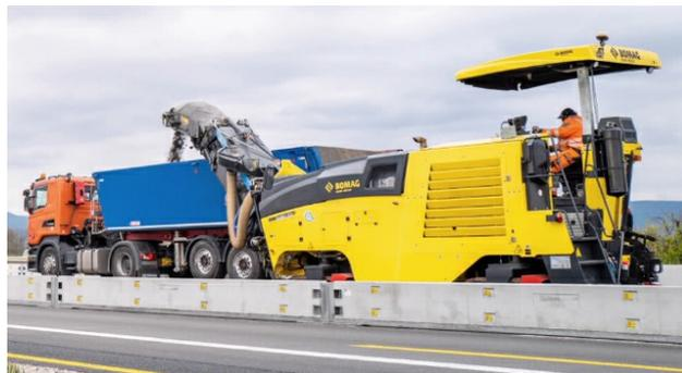
Bomag asphalt cold milling machine (Source: Data Panel)
