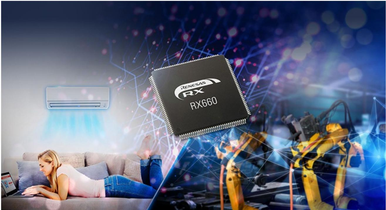
*The RX660 5-V and 32-bit MCUs with noise tolerance are suitable for home appliances and industrial applications (Source: Renesas)*
