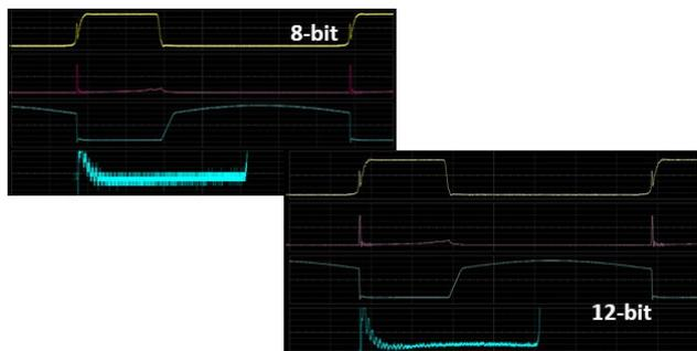
An 8-bit resolution acquisition shows a blurred saturation voltage trace with details buried in quantization noise but the 12-bit oscilloscope clearly shows details of the saturation voltage (Source: Siglent)
