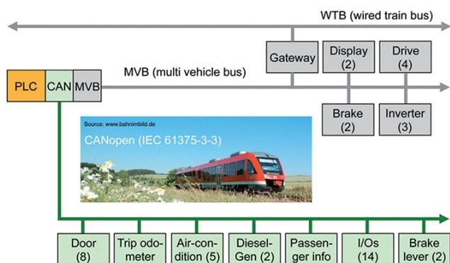
Figure 3: TCN architecture with CANopen (Source: CiA)
