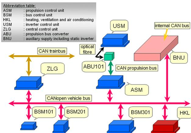
Figure 1: In-principle structure of the CAN-based networks within a vehicle
