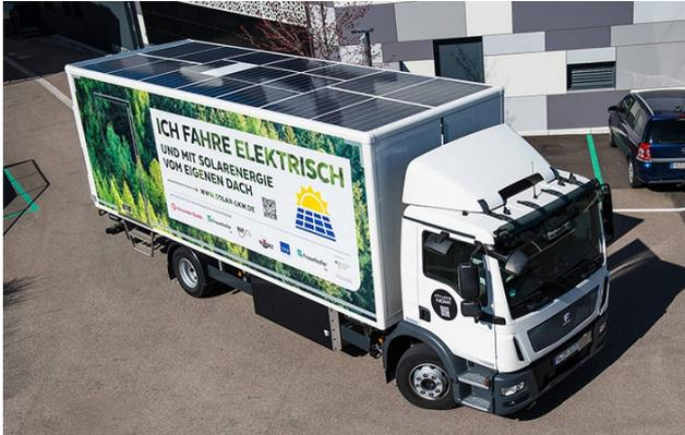
Figure 1: I drive electrically powered by photovoltaic on my roof (Source: Fraunhofer ISE)
