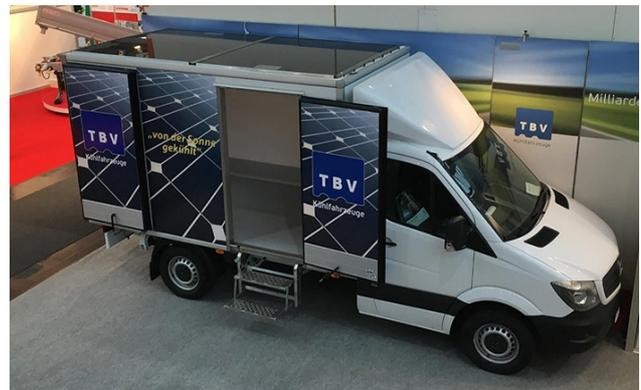
Figure 2: The refrigerated van from TBV uses integrated PV modules to support the refrigeration of the compartment (Source: TBV Kühlfahrzeuge)
