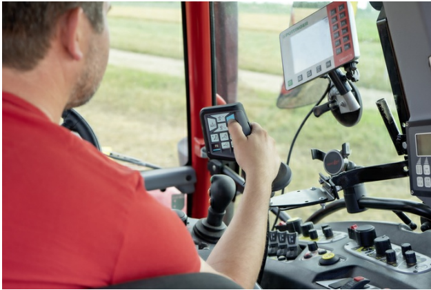
The Isobus joystick in action; it enables to control Isobus machines (Source: Poettinger)
