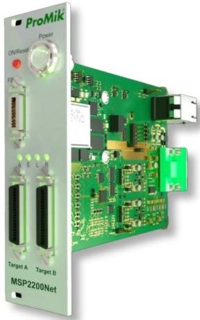
*The product is suitable for use of on-board programming and testing in electronic series production (Source: Promik)*
