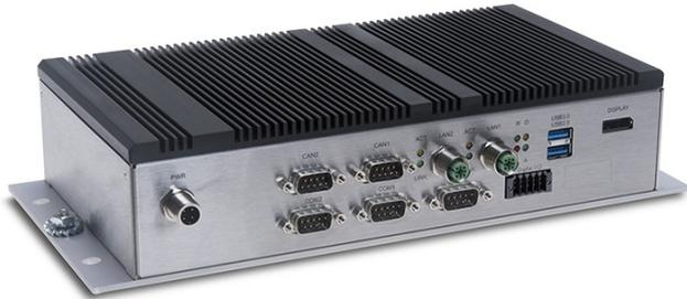
*The RML-R 82 supplements the portfolio of X86-based embedded systems for railway application (Source: Syslogic)*
